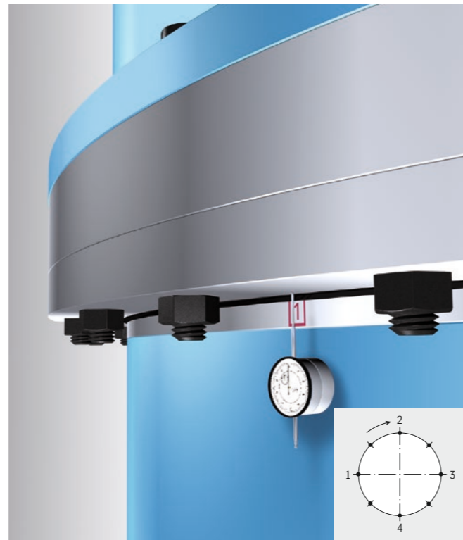
Figure 6: Basic setup for measuring the tilting clearance
