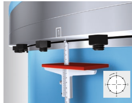
Figure 8: Basic setup for measuring the axial reduction with a depth gauge
